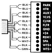
provided, install enclosure into wall. Strip jacket of 6pair cable 6" to identify the twisted pairs and assure correct connections. Strip insulation of each wire ¼" and connect to screw terminal in accordance with wiring diagram located inside enclosure.
